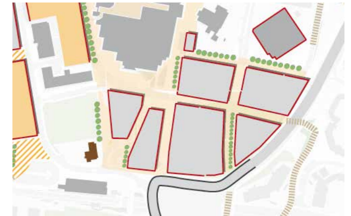
The framework for the area proposes a series of urban blocks and the establishment of a normal network of streets and spaces. The one-way loop of The Ring will be modified to create a normal two-way street including a new junction with Church Road to maintain access. Pedestrian and cycle connections are made more direct, improving the town-to-station links
